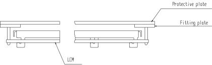
(2) When assembling the LCM into other equipment, the spacer to the bit between the LCM and the fitting plate should have enough height to avoid causing stress to the module surface, refer to the individual specifications for
