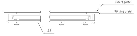
(2) When assembling the LCM into other equipment, the spacer to the bit between the LCM and the fitting plate should have enough height to avoid causing stress to the module surface, refer to the individual specifications for measurements. The measurement tolerance should be 0.1mm.
